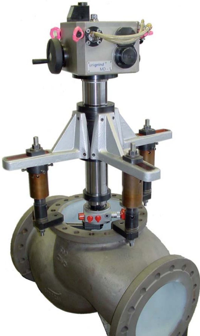
MD 1 Machining of globe valve seat
